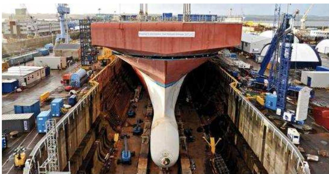
*The final bow unit to the carrier HMS Queen Elizabeth, completing assembly work on the forward part of the ship's hull – courtesy of the Aircraft Carrier Alliance, Spring 2013*
