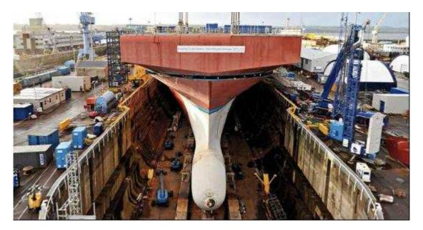
The final bow unit to the carrier HMS Queen Elizabeth, completing assembly work on the forward part of the ship's hull – courtesy of the Aircraft Carrier Alliance, Spring 2013
